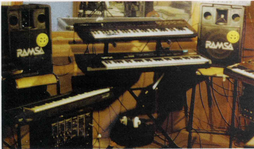
Richard Barbieri's keyboard rig: Roland System 700, Roland D50, Ensoniq VFX, Prophet 5, E-mu Emax
